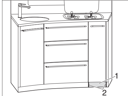
Fig. 109 Unscrewing skirting board
