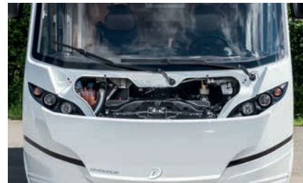
» I: Easy to service: large engine bay opening for servicing all relevant parts.
