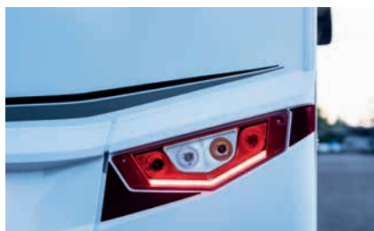
» T/I: Prominent and safe: Integral rear lights with LED night-time-running lights.
