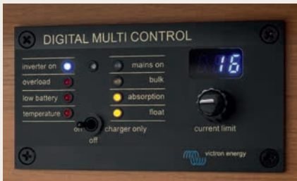
» Victron energy Digital MultiControl with control panel above the habitation door (optional)
