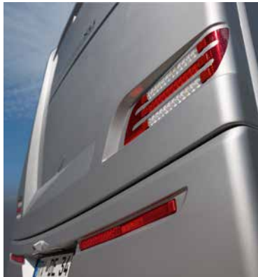
+ Repair-friendly: 2-piece GRP rear (1)
