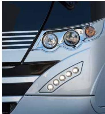
+ Two-piece GRP front with LED day-time-running lights (2)
