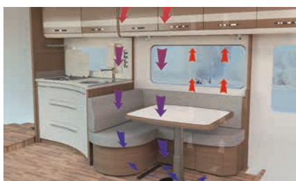
» AirPlus - perfect air circulation in the interior and ventilation behind the overhead lockers
