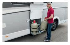
Comfortable: Extendable gas bottle locker for an easy change of gas bottles.
