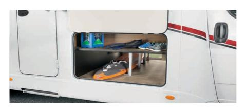
A 7877-2: High double floor with load-through possibility. Furthermore this vehicle basement is perfectly made for protecting the vehicle installations from cold temperatures.
