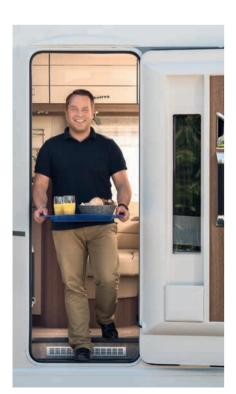
Extra wide entrance door (70 cm) with secure 2-point-locking system and central locking, window and flyscreen door.
