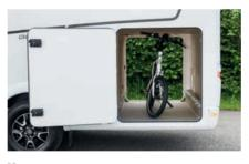
High and illuminated rear garage with 150 kg loading capacity and accessible from both sides. Two garage doors are standard.
